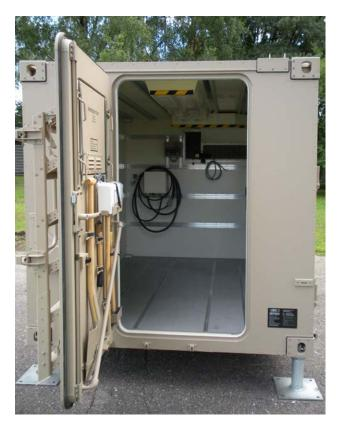
On request, the Aluminum-Shelter can be equipped with C-rails on the walls and in the floor for fastening the built-in parts.
